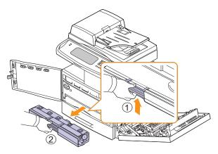
**5** Turn the imaging unit locking levers outwards to release and open the inner cover.
